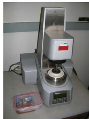
Rheometer for analysing the flow properties of faeces
