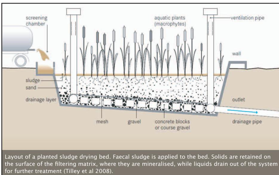
Layout of a planted sludge drying bed. Faecal sludge is applied to the bed. Solids are retained on the surface of the filtering matrix, where they are mineralised, while liquids drain out of the system for further treatment (Tilley et al 2008).
