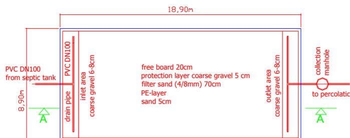
**Fig. 9:** Plan view of horizontal flow constructed wetland, flow is from left to right (source: EcoSan Club).
