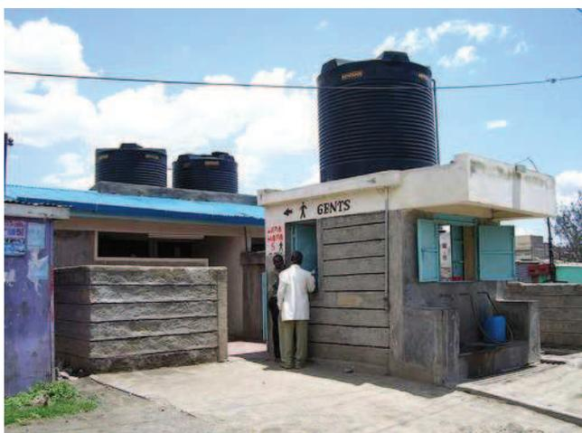
Figure 6: Naivasha public toilet with water kiosk. In front is the water kiosk that functions as an operator room. Customers pay at the side window, where the two people are standing. Behind them the gents section of the toilet can be seen (source: C. Rieck, 2008)<sup>3</sup>.
