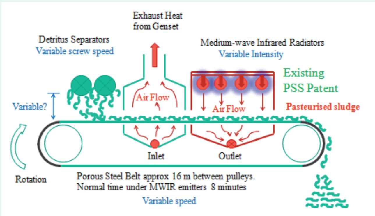
Figure 1 – Diagrammatic view of the LaDePa machine process
