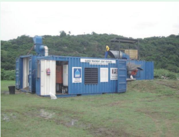
Figure 2 – The LaDePa machine assembled in a container.
