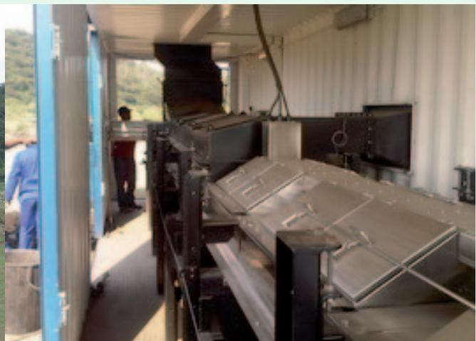
Figure 3 – The LaDePa machine inside the container.
