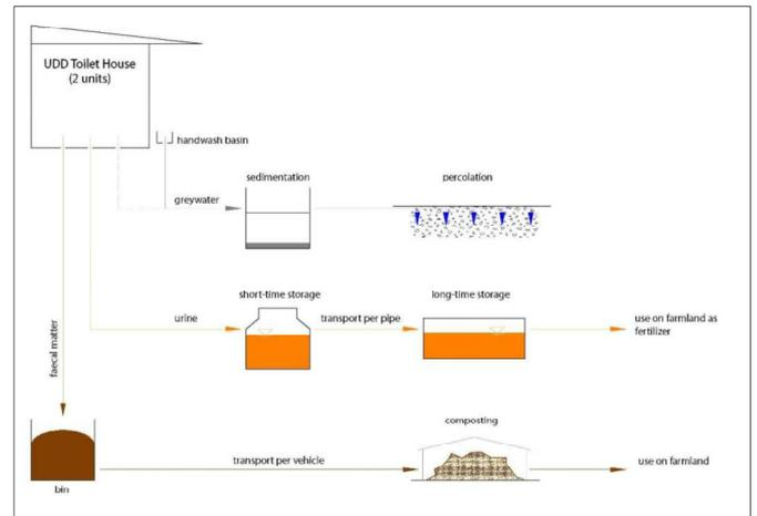
**Fig. 4:** Design of the UDDT system and treatment steps (source: Oldenburg et al. (2009)).
