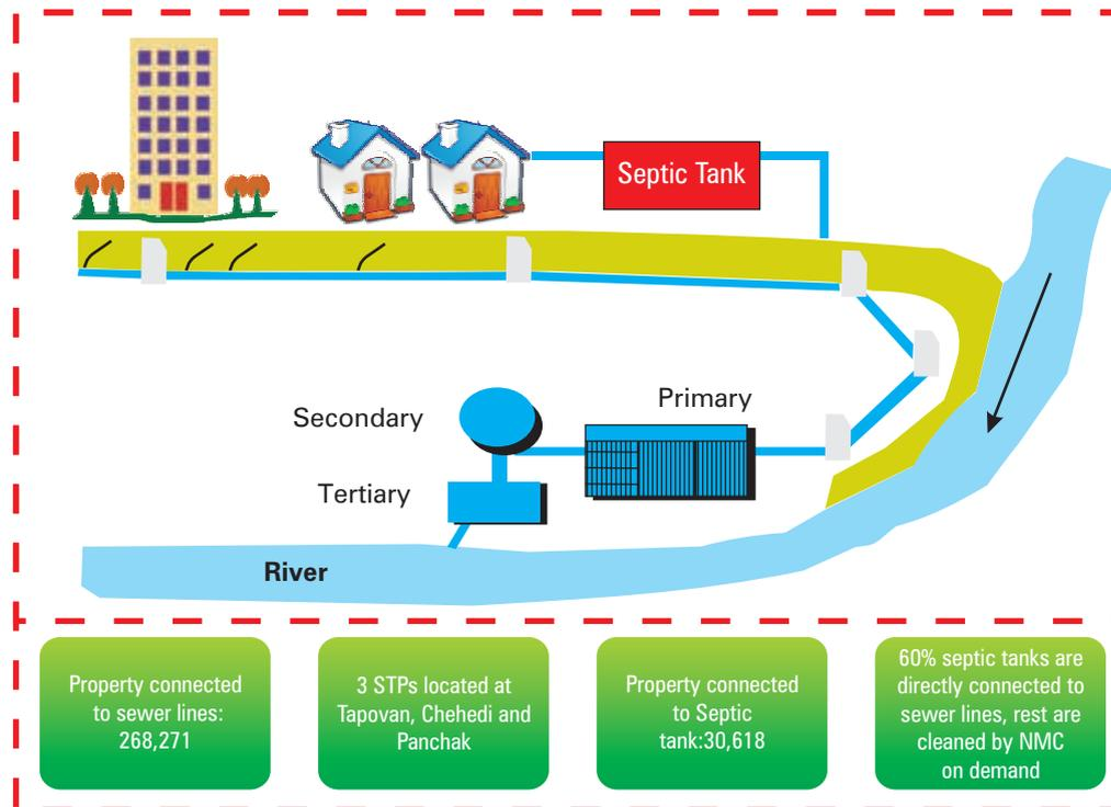
Figure 11: Schematic Diagram of Nashik's Sewerage System
