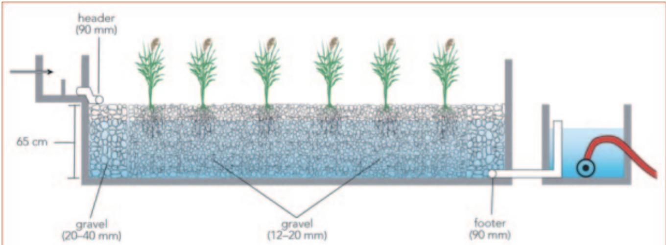
Figure 4: Secondary HF Wetland Cross Sectional View
