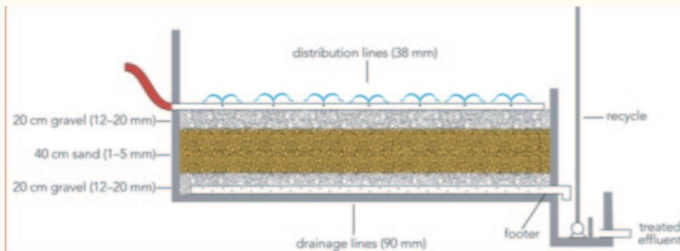
Figure 6: Tertiary VF Sand Filter Cross Sectional View
