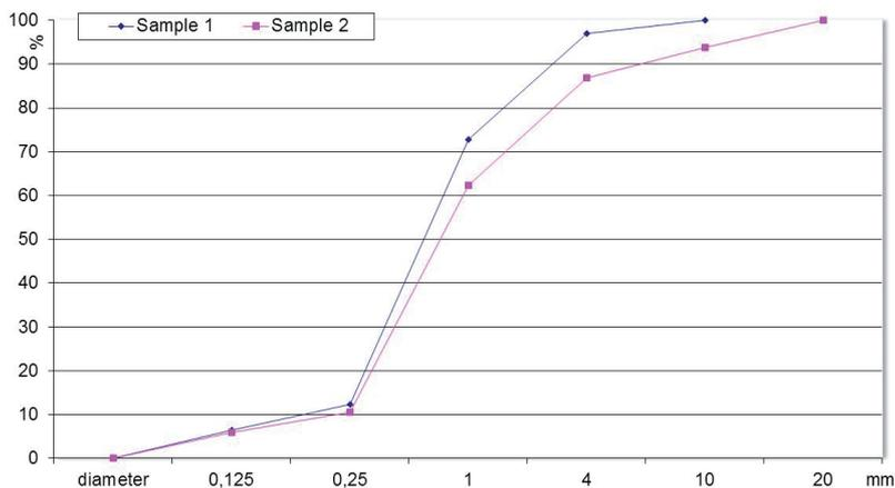
Figure 1: Sieve Analyses Filter Sand at Matany Hospital
