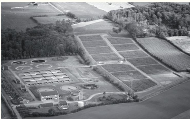
**Figure 1: Kolding Sludge Reed Bed System for 125000 PE (September 2000)**
