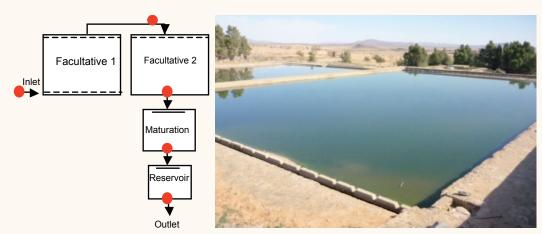
Figure 4. Flow diagram of Hammam Foukani's WSP, sampling points and view of the facultative ponds
