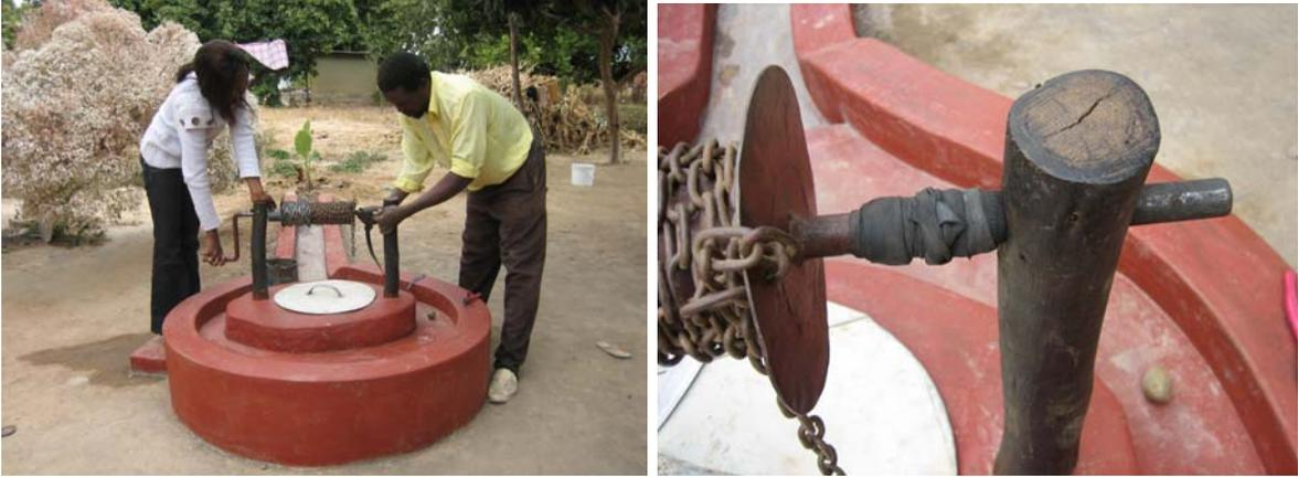
The windlass is mounted on the poles and is kept in position by attaching a length of rubber tubing around the windlass shaft. The windlass can be held in place in the slotted pole either with a nut and bolt passing through the pole or by nailing a piece of wood within the slot above the windlass shaft.
