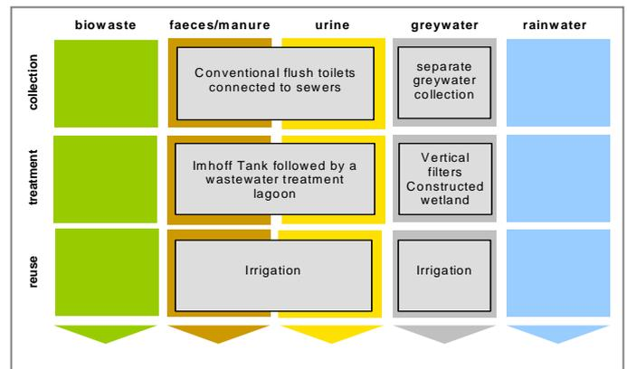
Fig. 2: Applied sanitation components of the overall project. (This case study focuses only on the greywater component.)
