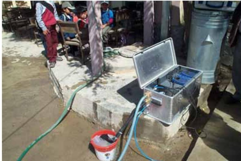
Figure 4: Continuous analysis of physicochemical parameters in a tube well in Kabul (T.TÜNNERMEIER)
