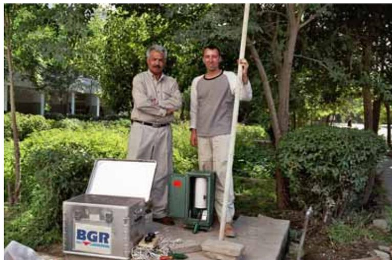
Figure 5: Installation of a groundwater level recorder in a tube well for the continuous observation of piezometric level variations (T.Krekeler)
