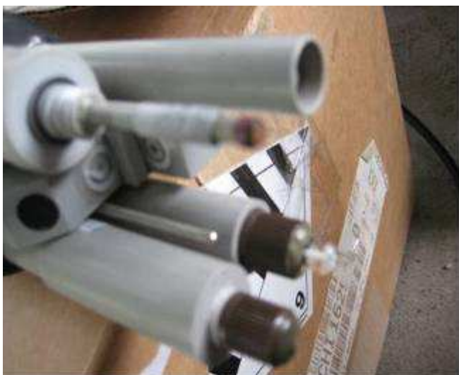
Figure 3-2 Checking probe of WQC – 22A (TOA-Japan), DO sensor was broken
