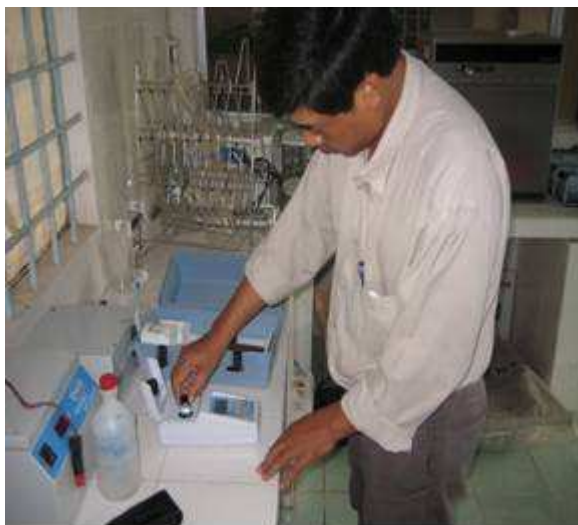
Figure 4-26 Measurement of turbidity in laboratory
