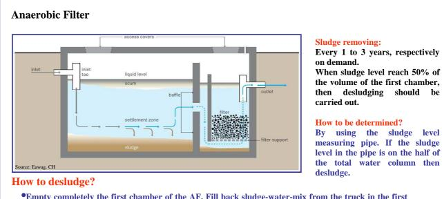
•Empty completely the first chamber of the AF. Fill back sludge-water-mix from the truck in the first chamber up to 30 cm height of the chamber. Fill up with water.
