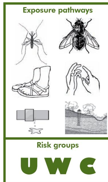
Lining is crucial. Furthermore the risk of groundwater contamination is also high (see exposure). The pit may also overflow and spread its contents to the surrounding areas.
