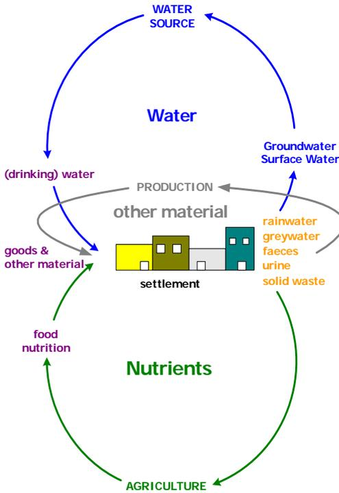
**Figure 1** Resource-oriented or ecological sanitation system (Langergraber and Müllegger, 2005)
