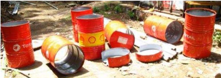
**Photograph 19 parts of the digester before welding**
