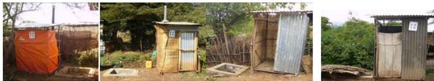
**Photograph 12 Fossa alternas constructed with different material**
