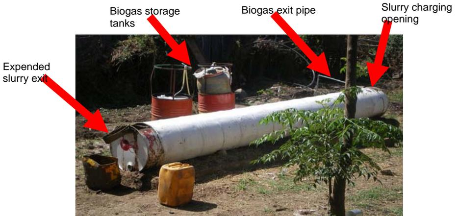
**Photograph 20 Parts of the digester after assembling all parts**
