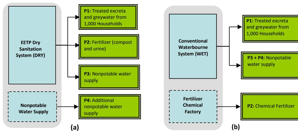
**Figures 5-1a and 1b.** System expansion of the (a) DRY and (b) WET systems as modeled in the LCA.
