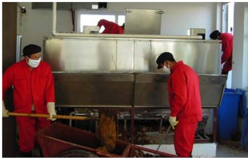
**Figure 7-12.** Sifting of materials from the faecal bins. [Source: Mertens, 2009.]
