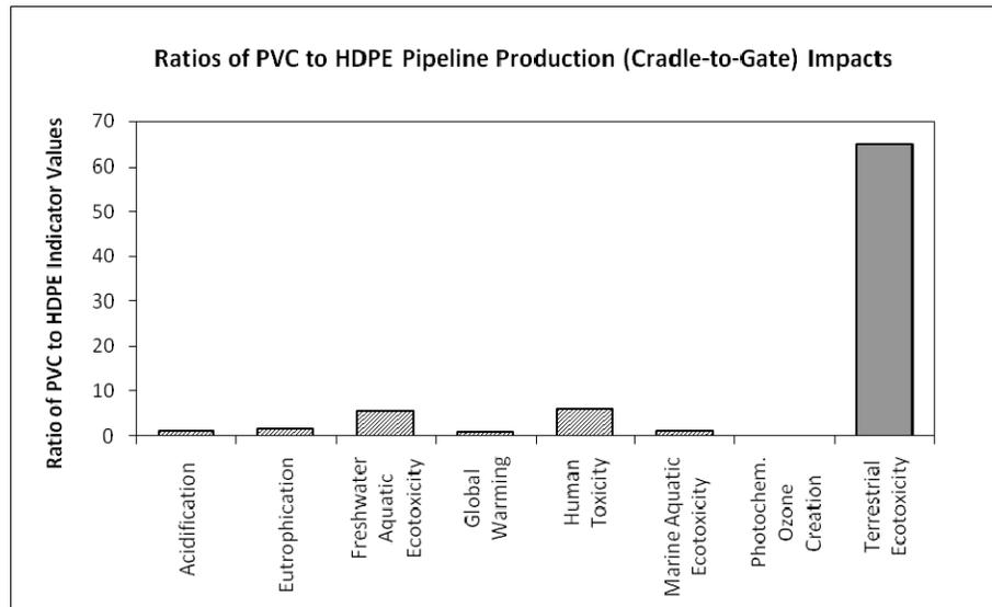
**Figure 8-2.** Ratios of the cradle-to-gate life cycle environmental impacts of one meter of 27-cm PVC pipeline versus HDPE pipeline.
