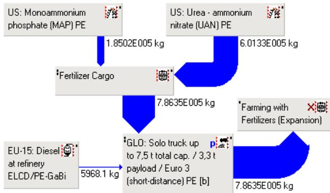
**Figure C-4.** GaBi LCA Plans: Operation of the Conventional Waterbourne System (WET System) and System Expansion (Fertilizer Supply) over a 20-Year Period.
