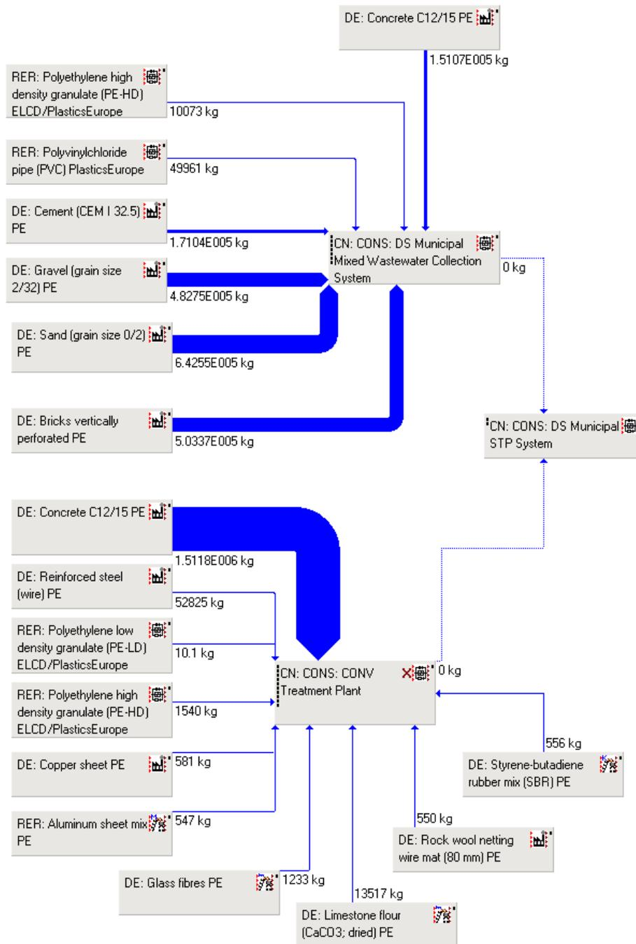
**Figure C-2.** GaBi LCA Plans: Construction of the Conventional Waterbourne System (WET System).
