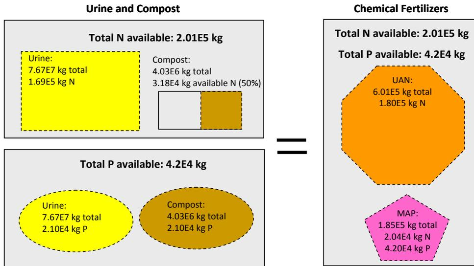
**Figure 5-6.** Components Included in the LCA: WET System – Fertilizer equivalents of urine and compost under system expansion (UAN: Urea- ammonium nitrate and MAP: monoammonium phosphate).
