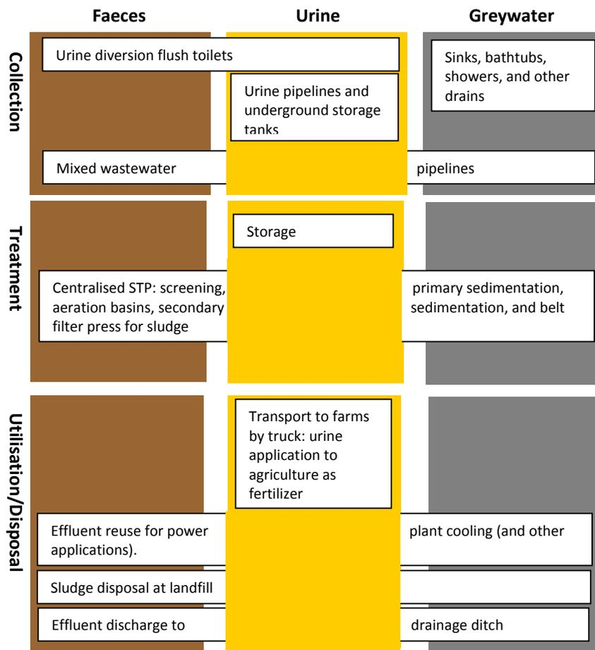
**Figure 9-3.** Alternative DRY System Scenario 2 (Alt-DRY-2) process schematic: Urine diversion with centralized treatment of blackwater and greywater at the Dongsheng STP.
