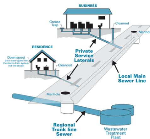
**Figure 7-15.** Illustration of a typical sewer system. The laterals carry one house’s or one building’s volume of wastewater, local mains carry a sub-area’s volume of wastewater, and trunk lines carry a region’s volume of wastewater. [Source: <http://www.ocwatersheds.com/>.]
