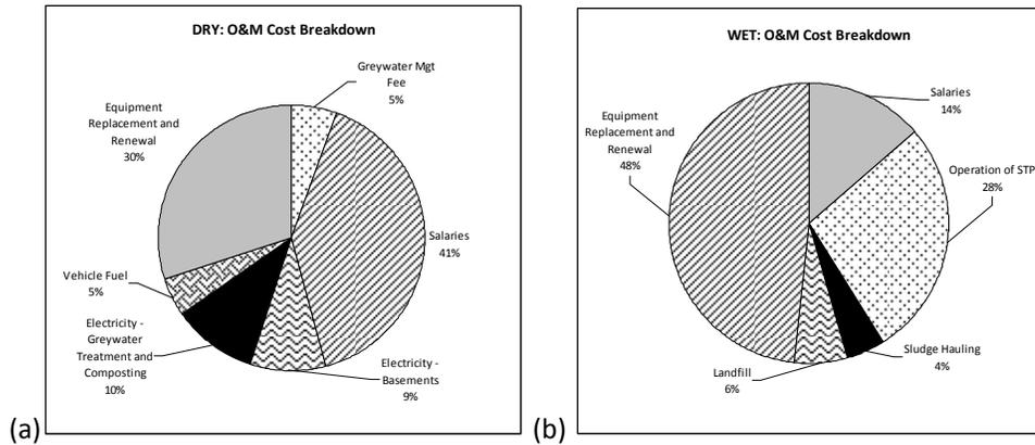
**Figures 6-3a and 3b.** Operation and Maintenance (O&M) cost breakdowns by item for the (a) DRY and (b) WET systems.
