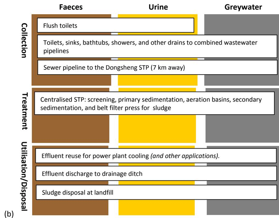
**Figures 3-10a and 3-10b.** The (a) DRY and (b) WET system scenarios and the associated collection, treatment, and utilization/disposal processes. Items in italics had not been fully implemented as of 2009.
