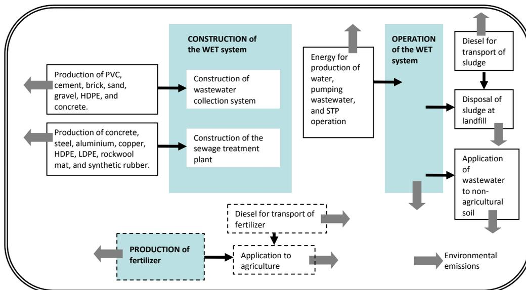
**Figure 5-3.** System boundary for the WET system LCA model. The dashed boxes represent system expansion.
