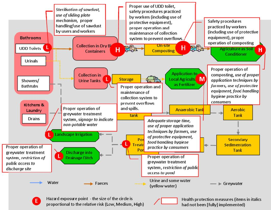
**Figure 7-8.** The hazard exposure points and associated health protection measures to reduce exposure and risk for the DRY system.
