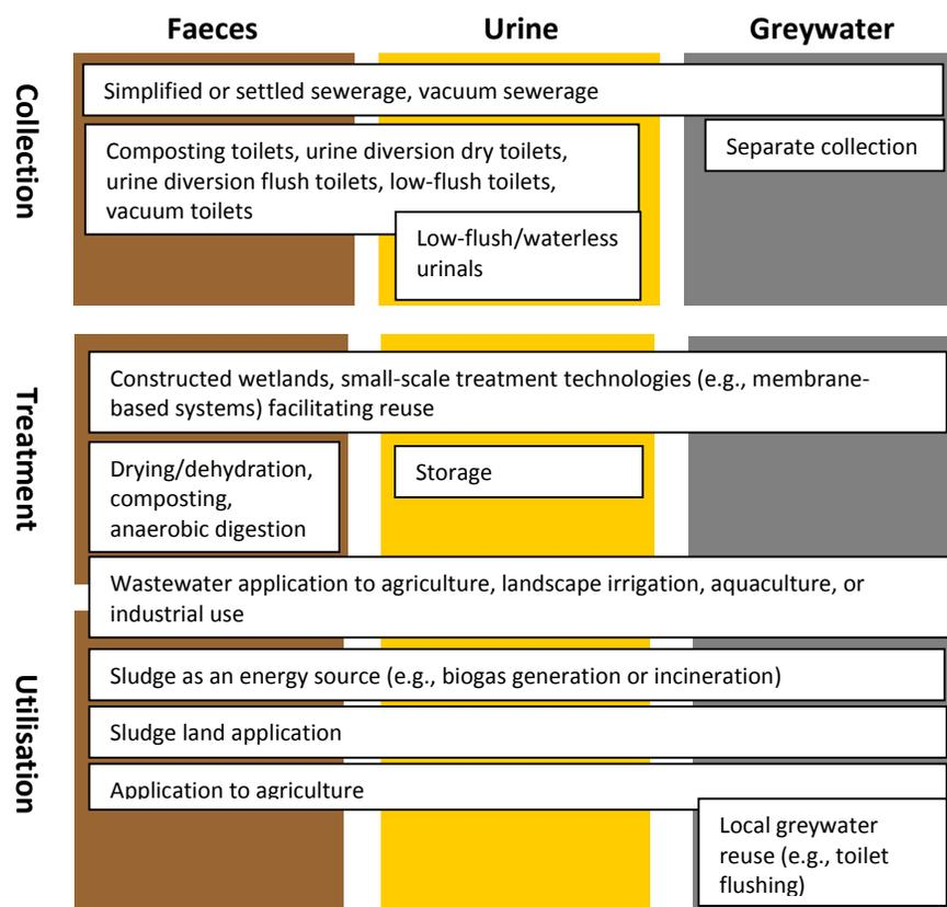
**Figure 2-1.** Examples of alternative (non-conventional) resource-oriented sanitation technologies (after UNESCO-IHP and GTZ, 2006).
