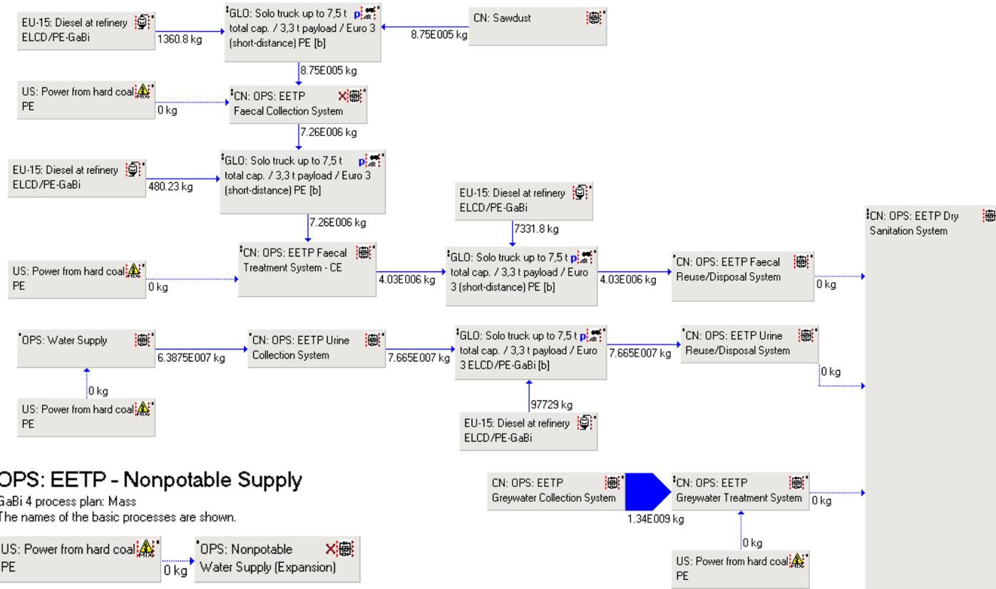
**Figure C-3.** GaBi LCA Plans: Operation of the EETP Dry Sanitation System (DRY System) and System Expansion (Nonpotable Water Supply) over a 20-Year Period.
