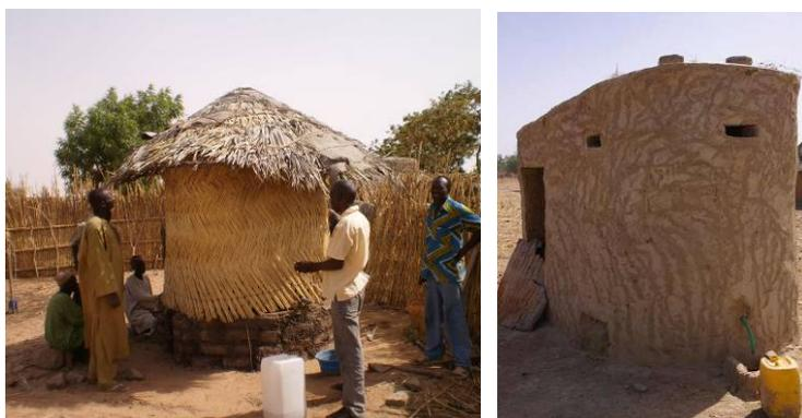
Different types of superstructure are possible, in straw or adobe for example. The roof is necessary to keep the vaults dry and to minimize the access to flies.
