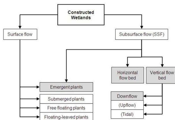
Figure 1. Classification of constructed wetlands (modified from Vymazal and Kroepfelová, 2008). The dashed ellipse signifies the focus of this document. HFB and VFB are abbreviations for horizontal and vertical flow bed, respectively. Hybrid systems are also possible. “Emergent plants” are a type of macrophyte where the leaves are *above* the water level.
