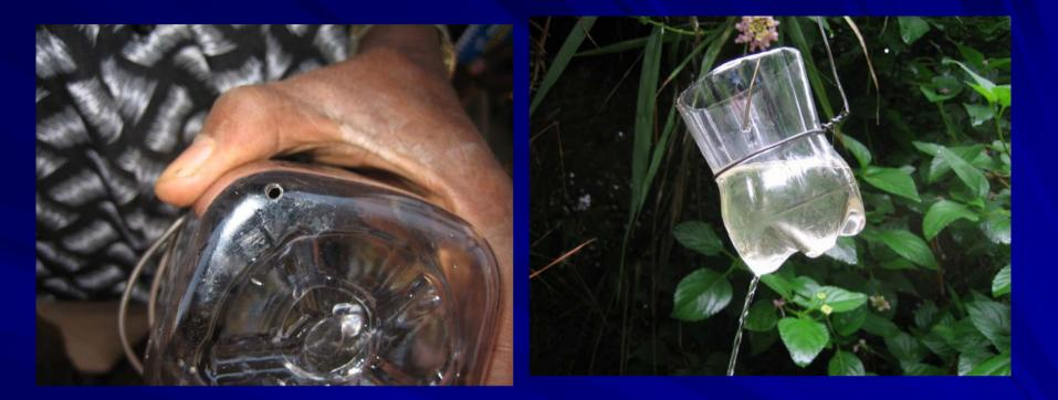
Wrap some thin wire around the bottle and hook up to part of the toilet. To use the washer it can be dipped into a container of water on the ground or some water from another bottle can be added to the washer. The water comes out slowly, but it is sufficient to wash the hands. It uses water economically. Tin cans can also be used. This is described next.
