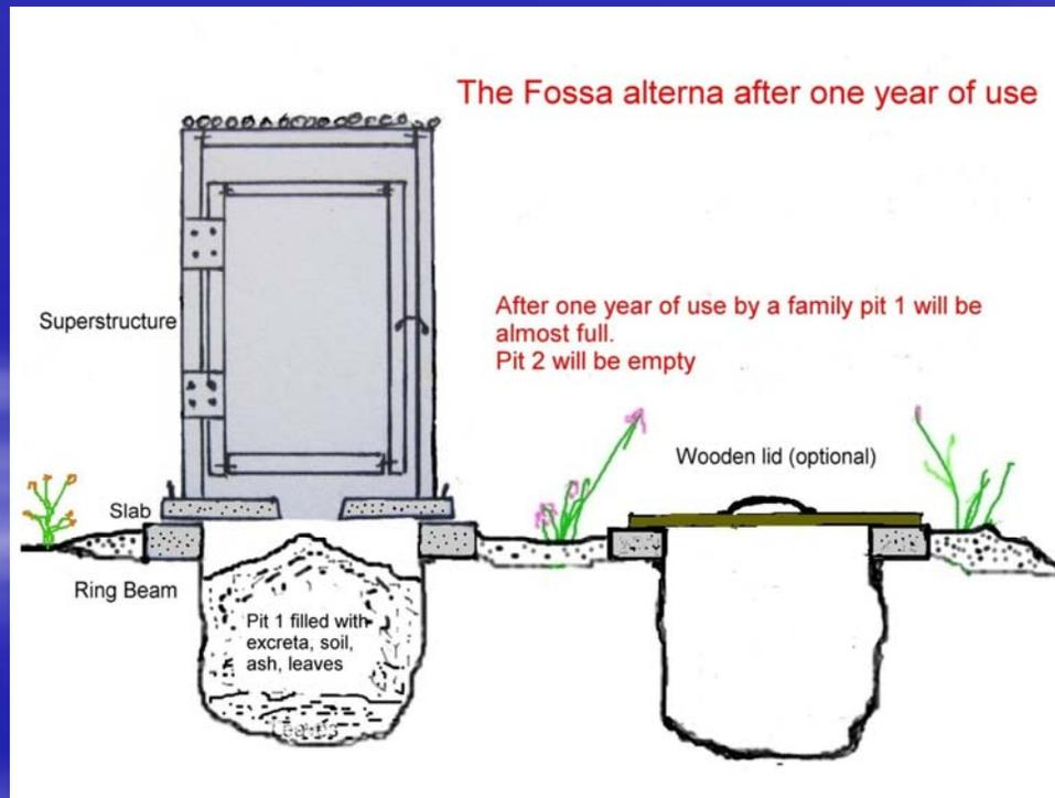
**Soil and wood ash are added frequently to the pit as well as excreta. This helps the composting process and helps to reduce flies and odours.**
