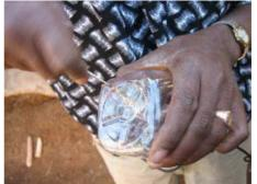
There are several types of simple hand washer. This one uses a plastic bottle. Cut the bottom off about one third up. Make a hole in one corner of the base.
