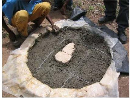
Figure 3-8: Cement and reinforcing wires in mould
