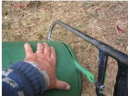
Figure 6-8: Cutting the base off the bucket
