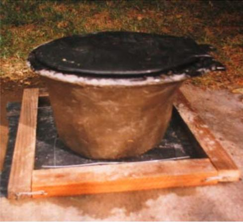
Figure 5-11: Completed pedestal placed in wooden mould
