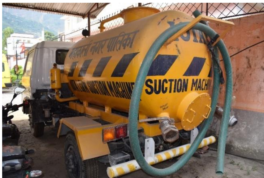
Figure 8: Desludging suction truck at Mahakali Municipality.
