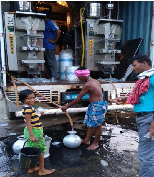
Figure 4: Provision of drinking water through mobile water treatment plant
