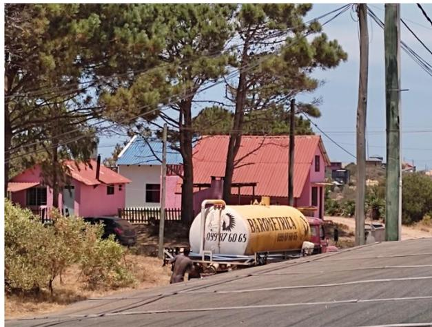
Figure 5: Vacuum truck equipped with a suction hose from the emptying service provider *El Indio* used to empty septic tanks. Source: (D&A and EP, 2021).
