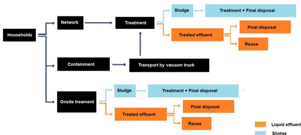
Figure 12: Simplified diagram of the sanitation configuration. Source: National Sanitation Plan.
