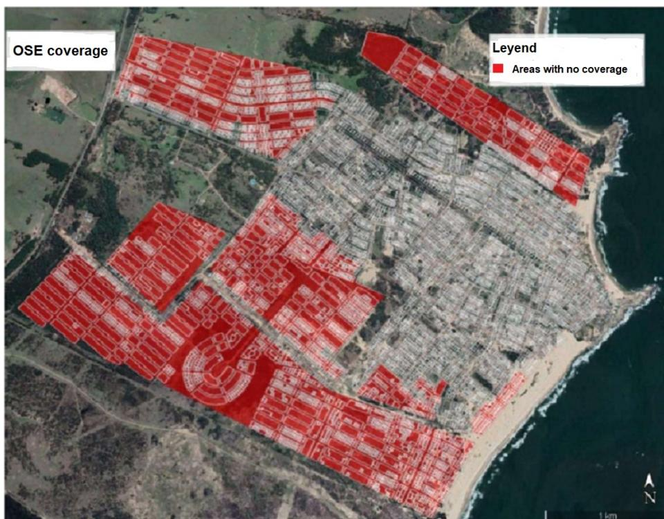
Figure 9: Sketch of OSE's drinking water distribution network. In red, the areas not covered by the distribution network. Source: (D&A and EP, 2021).
