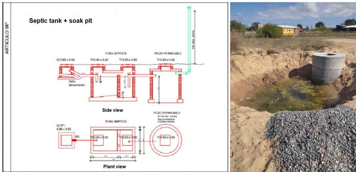
Figure 4: (Left): Sketch of the ordinance where the design of septic tanks is outlined; (Right): Septic tank under construction. Source: (D&A and EP, 2021).
