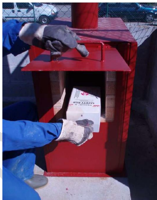
Figure 3: MSF Safety Box Reducer over a Sharps pit
