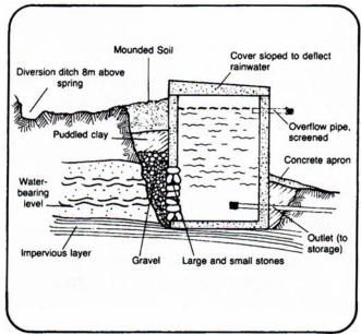
Figure 1: Spring box with single pervious side for hillside collection (Courtesy of USAID, 1982, available online at www.lifewater.org).
