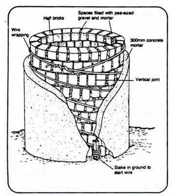
Figure 3: Spring box constructed with brick, wire and cement. (Courtesy of USAID, 1982, available online at www.lifewater.org).
