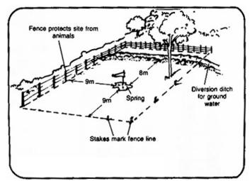
Figure 6: Preparation of spring box site (courtesy of USAID, 1982, available online at www.lifewater.org.)
