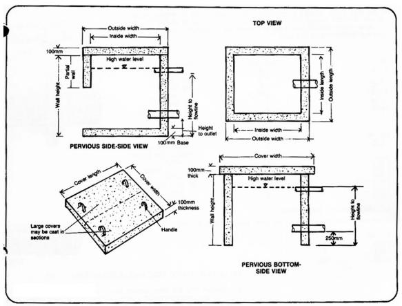
Figure 4: Dimensional plans of pervious side spring box and pervious bottom spring box (courtesy of USAID, 1982, available online at www.lifewater.org).
