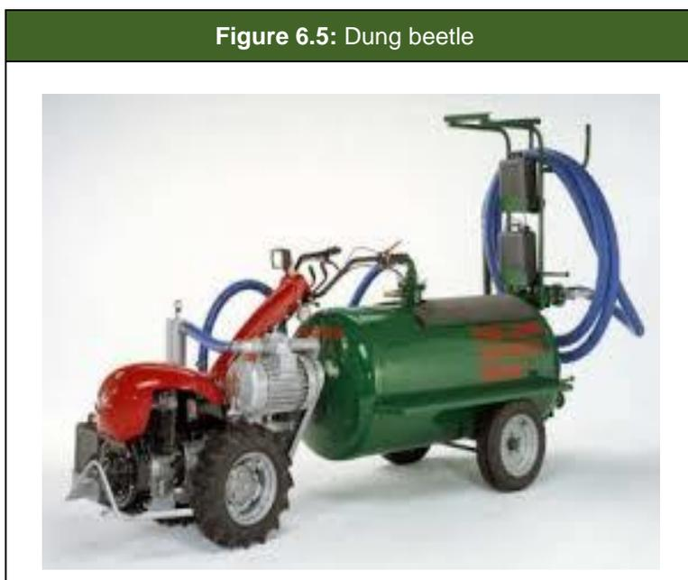
The sludge tank has a volume of approximately 800 litres and can create a maximum vacuum of 0.8 bar. The total weight when fully loaded, including that of the driver is approximately 1550 kg.
