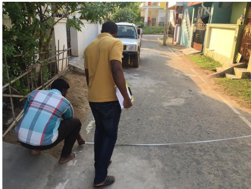
Figure A9.2: Measuring the Width of the Road to Observe the Truck Accessibility
