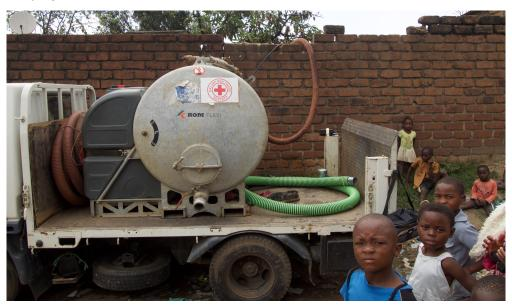
Figure 8. Mobile Desludging Unit (Source: Tilley, 2018)
