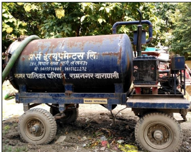
Figure 4: RNPP vacuum tanker used for emptying septic tanks/pits (Source: Shantanu/CSE, 2016)
