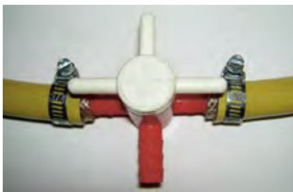
Picture 23: Model "Triple-valve" closed (left) and open (right) (photo: Sandec).
