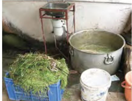
Picture 8: Electrical blender with water connection in India (photo: Sandec).
