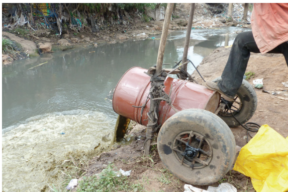
Figure 3: Manual emptier discharging the collected faecal sludge in a nearby stream ©GIZ/Doreen Mbalo
