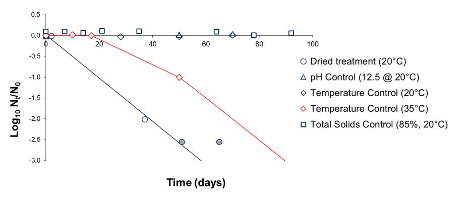
Log<sub>10</sub> inactivation of ascaris egg viability over time at 20 and 35°C in urine-Ca(OH)<sub>2</sub> suspension dried to a TS of 85% ( $\circ$ ) and controls for pH 12.5 ( $\Delta$ ) and TS 90% ( $\blacksquare$ ) and temperature ( $\Diamond$ ).
