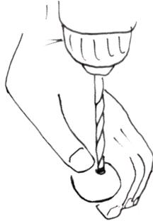
Drill a 1/4" hole in center of the bouncy ball.
