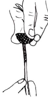
Screw the 6" long 1/4" toilet float rod or 1/4" screw stock into the bouncy ball.
