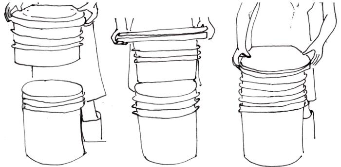
A cut off bucket becomes a flange to fit a seat tightly into a bucket.
