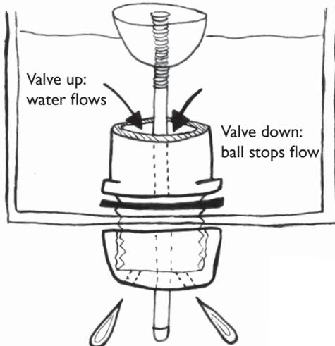
A quick tap from the back of the hand pushes the rod up, opening the valve.
