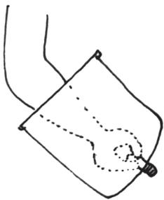
Screw 1" PVC threaded adapter through and out the bottom of the bucket.
