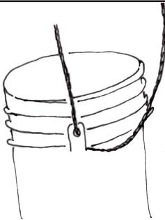
Run rope through the handle attachment hole on the lower bucket without the valve
