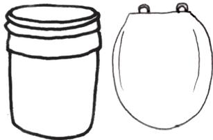
To make a toilet seat that can be fitted to buckets 3.5-7 gallons, take a 5 gallon bucket and cut the bottom off and screw the lip of the bucket into a toilet seat.
