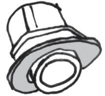
Stick 1" inner dia. rubber gasket around 1" PVC threaded adapter.
