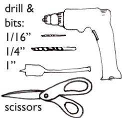
1/16" bit is for the water holes, 1/4" is to allow the tap rod through, and 1" cuts into the bucket.
