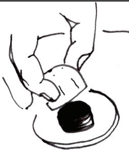
Screw 1" PVC end cap onto threaded adaptor. Tighten against the bottom of the bucket.
