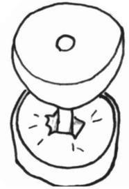
Put bouncy ball with toilet float valve screwed into it through the 1" PVC threaded adaptor.
