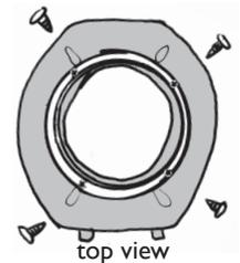
2. Place cut off bucket on top of the toilet seat so that the opening of the seat is entirely inside the bucket flange. Screw the cut off bucket into the toilet seat through the outer rim of the bucket., taking care not to screw through the wall of the bucket. Use four screws.
