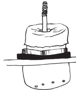
Pull cut glove over the top of the 1" PVC threaded adaptor so that it leaves an opening around the rod.
