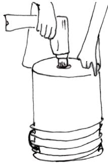
Drill a 1" hole in the bottom center of the bucket. Go slow and keep the drill level.
