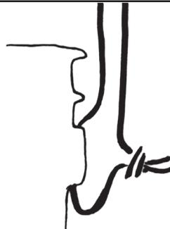
Run rope through the handle of the upper bucket (with valve) and tie off. Repeat on other side.
