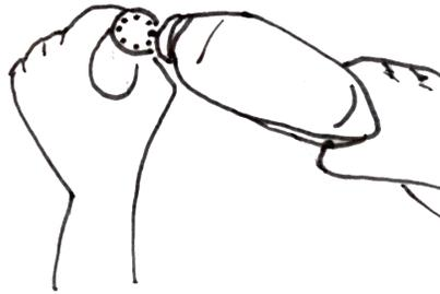
Hold PVC end cap in a clamp or wear gloves to protect your hands. Drill eight 1/16" holes for the water. Angle the drill out away from the middle of the cap.
