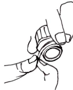
Wrap Teflon tape around the 1" PVC threaded adapter.
