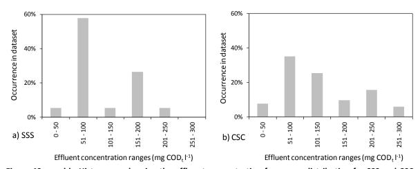
Figure 40 a and b: Histograms showing the effluent concentration frequency distribution for SSS and CSC system types
