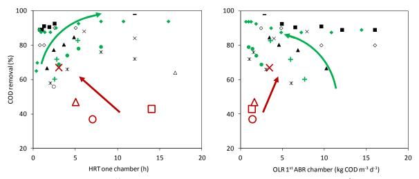
Figure 149: COD removal efficiency against one Figure 150: COD removal against 1<sup>st</sup> chamber OLR, chamber HRT, data from literature and case studies data from literature and case studies
