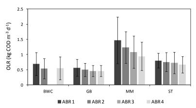
Figure 145: Biodegradable soluble OLRs of single ABR chambers of the four plants, error-bars indicate the standard deviation of COD₅ concentration measurements and a 20% variation of Q
