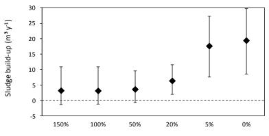
Fraction of intial hydrolysis rate constant used for model runs
