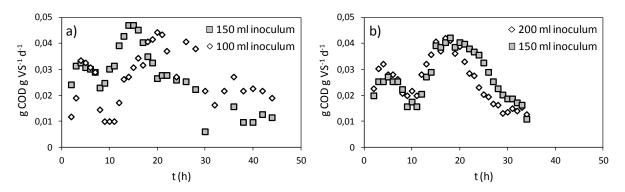
Figure 174 a and b: SMA curves of the experiments depicted in Figure 173, each data point represents the moving average over 4 h ( $t_i \pm 2$  h)
