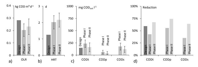
Figure 81 a, b, c and d: Loading and treatment parameters of the first five ABR chambers in Phase I and II: OLR, HRT, effluent COD concentrations and COD reduction rates, OLR error-bars indicate combination of standard error of mean of CODt measurements and standard deviation of Q, all other error-bars indicate standard deviations
