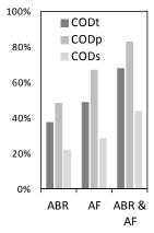
Figure 95: Average total, particulate and soluble COD profiles across reactor chambers as measured from 2009 to 2013, averages are calculated with 12 to 15 data points per sampling point, error-bars indicate standard deviations
