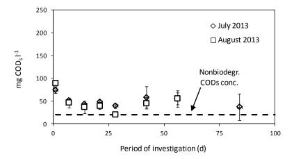
Figure 184: Nonbiodegradable effluent COD<sub>s</sub> concentration measurements done on samples taken at three different dates at ST (indicated as month and year), data-points represent the averages of single and duplicate measurements on duplicate samples, error-bars indicate the standard deviation of these three values
