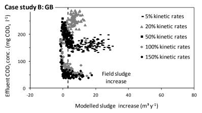
Figure 163: Sensitivity of the modelled effluent COD<sub>s</sub> concentration towards the hydrolysis rate and methanogenesis growth rate constant, modelling runs done with GB data
