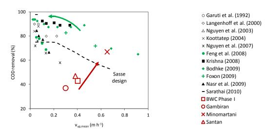
Figure 151: COD removal efficiency against average up-flow velocity  $v_{\text{up,mean}}$ , data from literature and case studies
