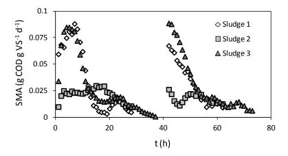
Figure 176: SMA curves of the experiments depicted in Figure 175, every data point represents the moving average over 4 h ( $t_i$  ±2 h)
