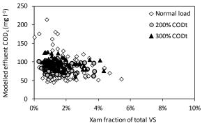
Figure 166: Xam fraction of total VS in reactor at the end of each modelling iteration vs modelled effluent COD<sub>5</sub> concentration depending on feed concentration
