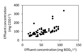
Figure 23: COD vs. BOD₅ effluent concentrations
