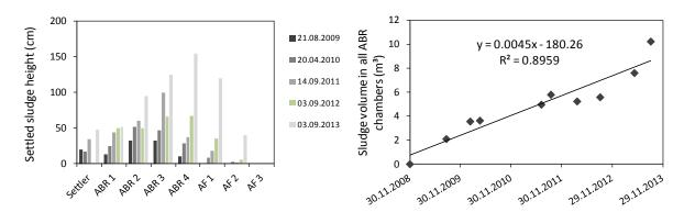
Figure 86: Selection of measured settled sludge levels in Gambiran
