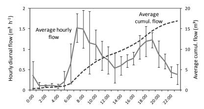
Figure 85: Average flows measured in 2009, averages were calculated with data from 07.08.2009 to 15.08.2009, error-bars indicate the standard deviation of hourly flows over this period
