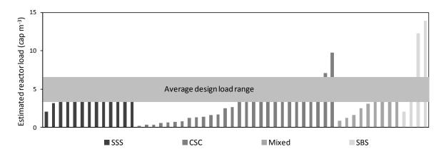
Figure 41: Loading estimation of plants (n = 54), the confidence range of the average design load is computed with the average load of 4.9 and the standard deviation of 1.6 cap  $m^{-3}$  (see Section 5.2.6)
