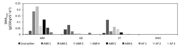
Figure 139: SMA<sub>max</sub> values measured across reactor chambers of three case study plants during dry-season
