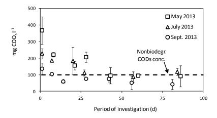
Figure 181: Nonbiodegradable effluent COD<sub>s</sub> concentration measurements done on samples taken at three different dates at BWC (indicated as month and year), data-points represent the averages of duplicate measurements on duplicate samples, error-bars indicate the standard deviation of these four values
