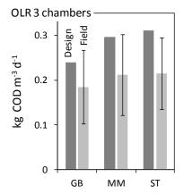
Figure 154: Average AF OLRs (three chambers) of three plants, error-bars indicate standard error of CODt conc. measurements and a 20% variation of Q
