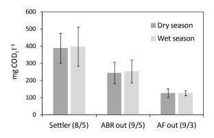
Figure 92: Average CODt concentrations measured at settler effluent, ABR effluent and AF effluent, "dry season" is defined as the months May to September, "wet season" is defined as the months October to April, the numbers in brackets indicate the number of measurements made during dry and wet season respectively
