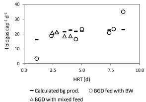
Figure 25: Cumulative biogas production over three to four days measured at six plants
