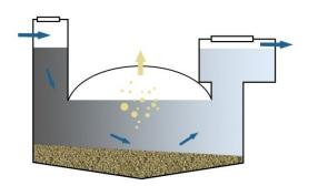
Figure 4: Cross section of a typical BORDA fixed dome biogas digester (courtesy of BORDA)
