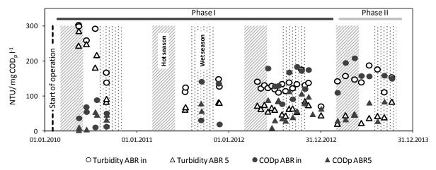
Figure 77: ABR<sub>in</sub> and ABR 5 turbidity and COD<sub>p</sub> concentrations, the light red areas indicate the warmest period of the year, the light blue areas indicate the wettest period of the year
