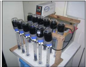
Figure 170: Conceptual representation of the SMA setup with temperature controlled water-bath, reactor bottle, displacement bottle and measurement cylinder, adapted from Pietruschka (2013)
