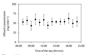
Figure 24: Average hourly effluent COD-concentrations from hourly measurements done on five consecutive days from the 19<sup>th</sup> to the 23<sup>rd</sup> of July, 2008 in Minomartani, Indonesia, error-bars indicate the standard deviation of hourly measurements (Reynaud, 2008)
