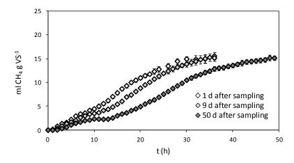
Figure 177: Cumulative CH<sub>4</sub> production at constant substrate (NaAc) concentration (1 g COD l<sup>-1</sup>), constant inoculum (sludge) volume (150 ml) and varying storage times, data-points are averages of triplicates and control has been subtracted, error-bars indicate the sum of standard deviations of triplicate tests and triplicate controls, the theoretical maximal CH<sub>4</sub> production is 20 ml CH<sub>4</sub> g VS<sup>-1</sup>, sludge sample: ABR 1, Minomartani
