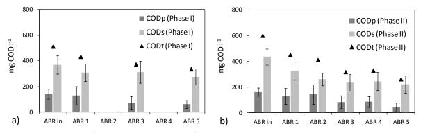
Figure 79 a and b: COD fraction concentration profiles as measured in reactor chambers, error-bars indicate standard deviations
