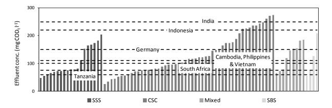
Figure 39: Effluent  $COD_t$  values at visited plants not affected by rain water and with raw-water conductivity below 6 mS cm<sup>-1</sup> (n = 82), the dotted red lines represent national standard discharge COD concentration values for various countries
