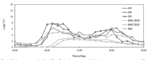
Figure 21: Average per capita diurnal flow fluctuations measured during six measurement campaigns at five sites
