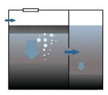
Figure 5: Cross section of a typical setter or septic tank (courtesy of BORDA)
