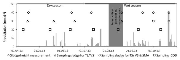
Figure 68: Precipitation data and sludge sampling and height measurement dates in Phase II
