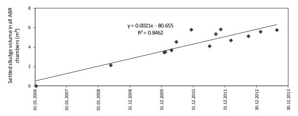
Figure 105: Total ABR sludge volume accumulation in Minomartani
