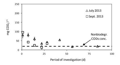
Figure 182: Nonbiodegradable effluent COD<sub>s</sub> concentration measurements done on samples taken at three different dates at GB (indicated as month and year), data-points represent the averages of single and duplicate measurements on duplicate samples, error-bars indicate the standard deviation of these three values
