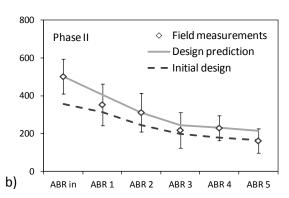
Figure 82 a and b: Measured average CODt concentration profiles in Phase I and II, initial design predictions ("Initial design") and design predictions with input variables adjusted to measured field values ("Design prediction")
