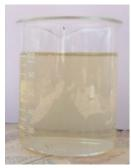
Figure 35: Sample with measured COD concentration of 1,649 mg CODt l<sup>-1</sup>
