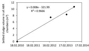
Figure 119: Measured settled sludge levels in Santan
