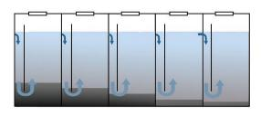
Figure 6: Cross section of a five chamber ABR (courtesy of BORDA)
