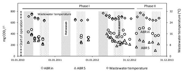
Figure 78: ABR<sub>in</sub> and ABR 5 COD<sub>s</sub> concentrations and measured wastewater temperature, the light red areas indicate the warmest period of the year, the light blue areas indicate the wettest period of the year
