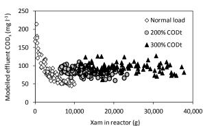
Figure 164: Xam in reactor at the end of each modelling iteration vs modelled effluent CODs concentration depending on feed concentration
