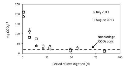
Figure 183: Nonbiodegradable effluent COD<sub>s</sub> concentration measurements done on samples taken at three different dates at MM (indicated as month and year), data-points represent the averages of single and duplicate measurements on duplicate samples, error-bars indicate the standard deviation of these three values
