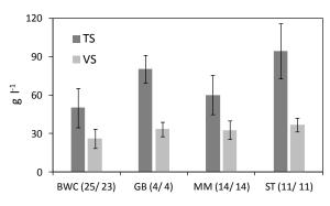
Figure 135: Average ABR settled sludge TS and VS concentrations at the four sites, error-bars indicate standard deviations of measurements across chambers
