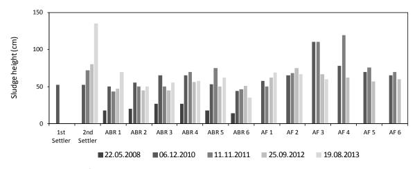
Figure 104: Selection of measured settled sludge levels in Minomartani
