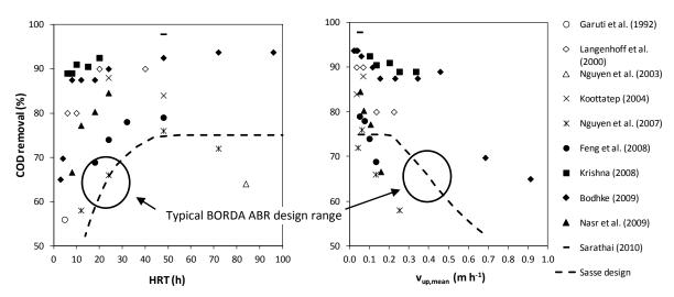
Figure 11: Performance efficiency against various hydraulic retention times
