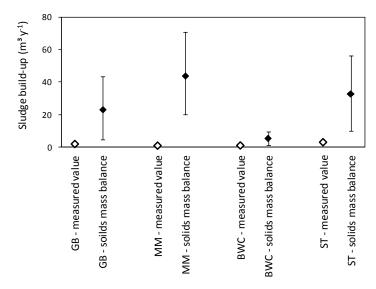
Figure 146: Average sludge build-up rates observed in reactors and estimated through mass balance of particulate organics, error-bars represent confidence intervals taking a feed flow variation of 20%, the standard error of means of COD<sub>p</sub> concentrations and the standard deviation of sludge VS concentration data into account
