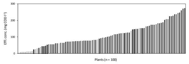
Figure 38: Effluent CODt concentrations and rain occurrence prior to sampling (light columns represent sites where it rained within 24 h prior to sampling) at visited plants with raw-water conductivity below 6 mS cm<sup>-1</sup> (n=100)
