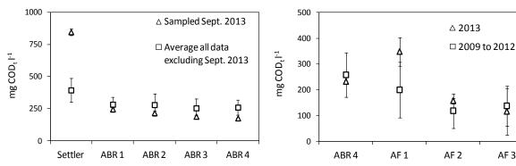
Figure 93: CODt concentration profiles across ABR Figure 94: Comparing CODt concentration profiles across AF chambers measured in 2013 and before chambers and outlier value measured in September 2013
