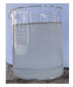
Figure 37: Sample with measured COD concentration of 416 mg CODt I<sup>-1</sup>
