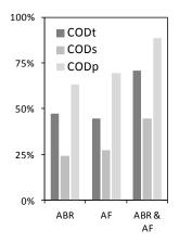
Figure 127: Average total, particulate and soluble COD profiles across reactor chambers as measured from 2011 to 2013, averages were calculated with 9 to 10 data points per sampling point, error-bars indicate standard deviation
