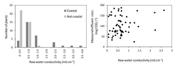
Figure 48: Histograms for the raw-water Figure 49: Raw-water conductivity and effluent conductivity frequency distribution depending on concentration whether a plant is built in a coastal area or inland
