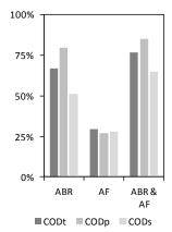
Figure 111: Average total, particulate and soluble COD profiles across reactor chambers as measured from 2010 to 2013, averages were calculated with 6 to 12 data-points, error-bars indicate standard deviations
