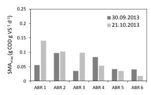
Figure 72: SMA<sub>max</sub> values of sludge sampled from different reactors in 2013 at BWC, all sludges were processed within one week after sampling, all values were derived from single measurements
