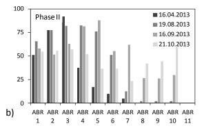
Figure 69 a and b: Selection of settled sludge levels measured in Beedi Workers Colony, Phase I and II
