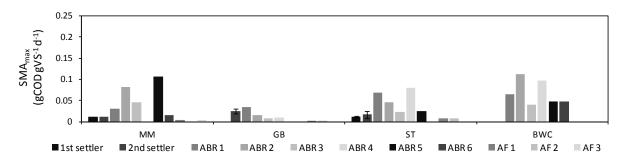
Figure 138: SMA<sub>max</sub> values measured across reactor chambers of the four case study plants during wet-season
