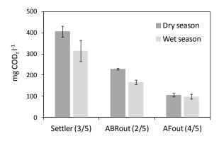
Figure 125: Average CODt concentrations measured at settler effluent, ABR effluent and AF effluent, "dry season" is defined as the months May to September, "wet season" is defined as the months October to April, the numbers in brackets indicate the number of measurements made during dry and wet season respectively
