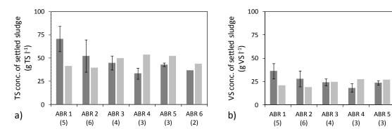
Figure 71 a and b: Settled sludge TS and VS average concentration profiles, number of measurements in brackets, error-bars indicate standard deviations of multiple measurements
