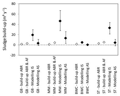
Figure 159: Average sludge build-up rates in m³ y⁻¹, field data (not full), modelled data (full), error-bars of full data points represent 95% confidence intervals of modelled outcomes after Monte-Carlo type uncertainty analysis taking into account the measured uncertainties of model input data
