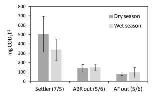
Figure 110: Average CODt concentrations measured at settler effluent, ABR effluent and AF effluent, "dry season" is defined as the months May to September, "wet season" is defined as the months October to April, the numbers in brackets indicate the number of measurements made during dry and wet season respectively
