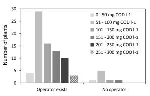
Figure 51: Histograms for the effluent concentration frequency distribution depending on operator existence
