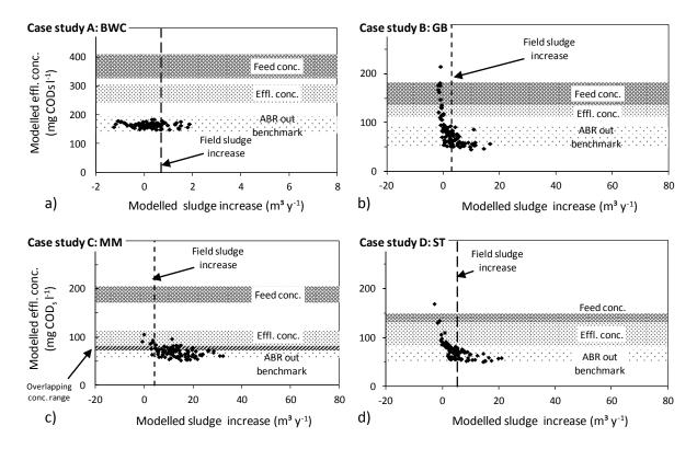
Figure 162 a, b, c and d: Modelled sludge increase representing active anaerobic treatment vs. effluent COD<sub>s</sub> concentration. The red and blue horizontal bands represent the 95% confidence intervals of measured feed and effluent COD<sub>s</sub> concentration means respectively, the grey horizontal band highlights the benchmark effluent COD<sub>s</sub> concentration given by the model
