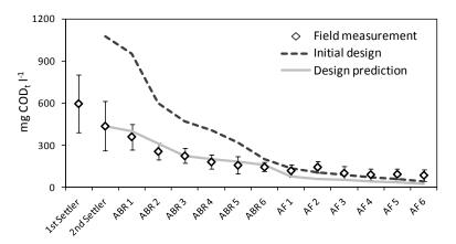
Figure 114: Measured average CODt concentration profile, initial design prediction ("Initial design") and design prediction with input variables adjusted to measured field values ("Design prediction")
