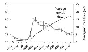
Figure 64: Average flows measured in 2012, averages were calculated with data from 8 d (23.04.2012 to 30.04.2012)
