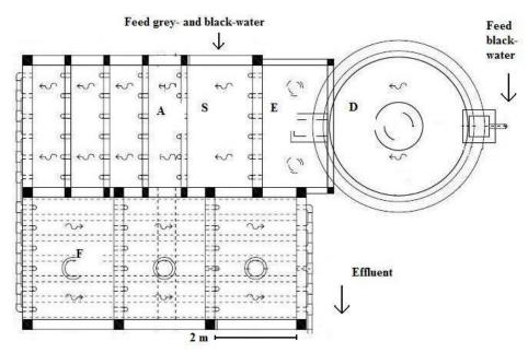
Figure 83: Schematic diagram (top-view) of the DEWATS plant built in Gambiran/ Yogyakarta with biogasdigester (D), expansion chamber (E), settler (S), ABR (A), anaerobic filter (F); water-depth of the system: 2,000 mm
