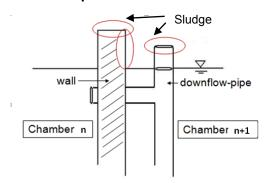
Criteria for exposure of an ABR to storm water were observations such as sludge on partition walls or on down flow pipes as shown in Figure 14.
