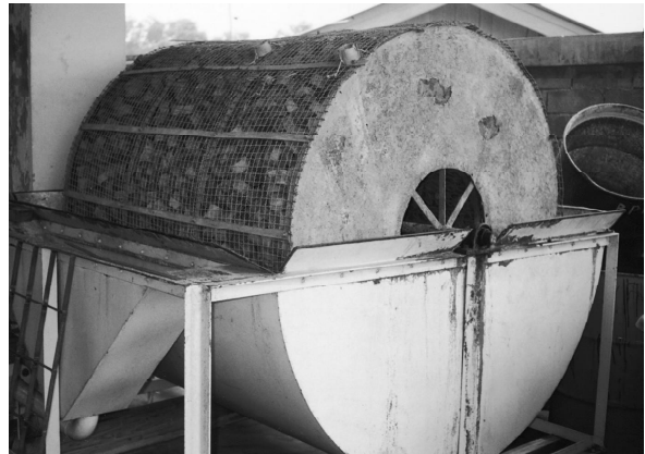
Fig. 52. Rotating disk reactor in a slaughter house in Jakarta, Indonesia. The reactor was temporarily out of use when the photograph was taken. [photo: Sasse]
