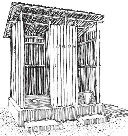
Figure 9.3. Pour-flush pit latrines
