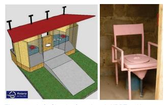
**Figure 57**. Left: Sketch of two bench UDDTs with a ramp for a public toilet in Peru, which could easily be modified with handrails and handlebars to increase accessibility for people with disabilities (source: *Rotaria del Peru SAC*, 2010). Right: A metal chair is used to hold a UD insert for use by elderly people in Burkina Faso (photo: M. Fogde, 2010).
