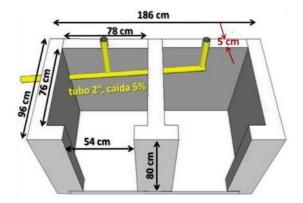
**Figure 20.** Sketch of double dehydration vaults with dimensions for a bench design like the one in Figure 19. The vault volume is about 500 litres each (source: Hoffmann, 2012). Tubo 2" is Spanish and means pipe with diametre of 2 inches and 'caida' means slope (%5).
