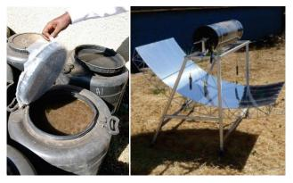
**Figure 42**. Left: Urea treatment of faecal sludge from pit latrines in Kampala, Uganda (photo: E. v. Münch, 2012). Right: Solar concentrator by *Sanivation* heating faecal matter from UDDTs in a black drum in Chile (photo: A. Foote, 2010).
