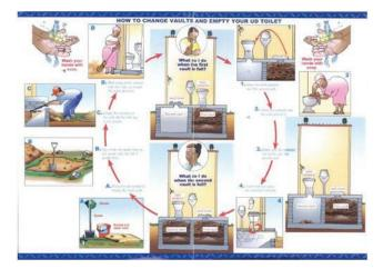
**Figure 47**. Instructional poster depicting how to switch between vaults and empty dehydrating vaults from eThekwini Municipality, South Africa (source: Roma et al., 2011).
