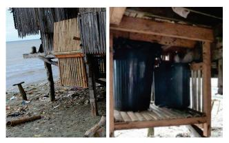
**Figure 61**. A hanging single vault urine-diverting dry toilet at a shore line area in the Philippines<sup>44</sup> (photos: R. Gensch, 2010).
