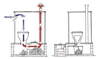
**Figure 16**. A double dehydration vault UDDT (left) with the indication of the air flow through the ventilation pipe, and a single vault with interchangeble containers (right) (source: M. Morgan, 2007). There can also be one ventilation pipe for each dehydration vault (see Section 4.9).
