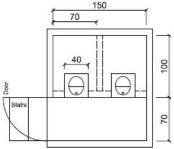
UDDT with single drop hole pan (single vault)
