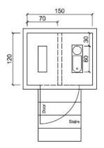
UDDT with twin drop hole squatting pan (double vault)
