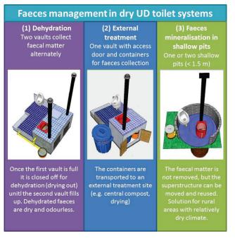
Figure 1. Overview of three different faeces management methods for UDDTs (Hoffmann, 2012).
