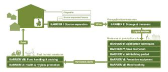
**Figure 36**. Multi-barrier concept for safe use of urine as a fertiliser (source: Richert et al., 2010)
