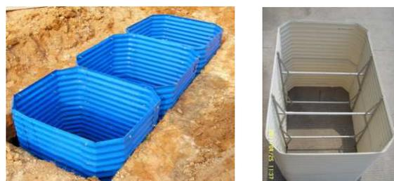
Figure 7: Emergency pit lining kits to avoid collapse. A man hole provides access for desludging. Left: modular corrugated plastic. Right: new design with internal props (instead of relying on locally available wooden props included in former design (source: J. Rhode, Evenproducts, 2011).
