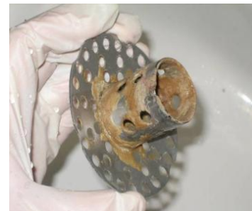
Fig.14: Urine scale deposition on a waterless urinal's outlet sieve (old model) (source: L. Ulrich, December 2008). With the new model of the sieve and rubber tube seal (see Fig. 9 right), such urine scale formation and internal pubic hair accumulation is reduced.
