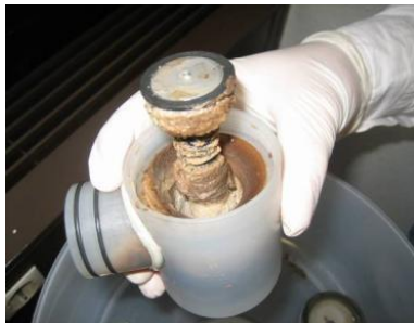
Fig.15: Soft urine precipitations inside a urine valve of a Roediger urine-diversion toilet. This valve was disassembled and cleaned after clogging (source: L. Ulrich, December 2008). One valve costs EUR 118 and requires a bowden cable costing EUR 51 (location of valve in Fig. 9).
