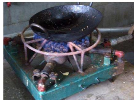
fig. 7: Use of biogas as substitute to LPG in cooking. (source: seecon gmbh)
