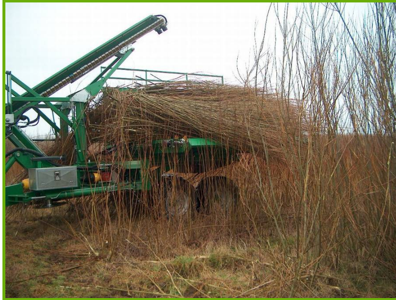
Picture 18. Nordic Biomass Stemster MK II harvesting in a willow SRP. [Photo by: Nordic Biomass]
