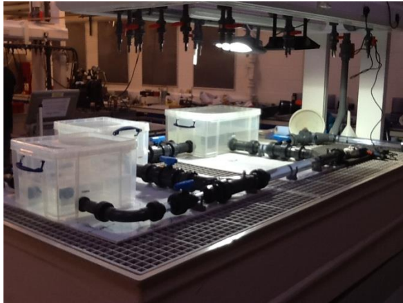
Small scale Voraxial SP2 (2 way liquid-liquid separation)
