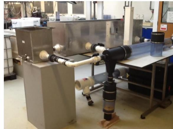
Larger scale Voraxial BD2 (3 way liquid-liquid-solid separation)
