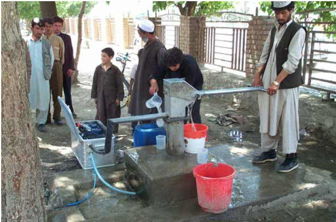
Fig. 2.2: Sampling a well in the city of Kabul. The well outflow is connected to the measuring equipment by a rubber hose (photo: TÜNNERMEIER).
