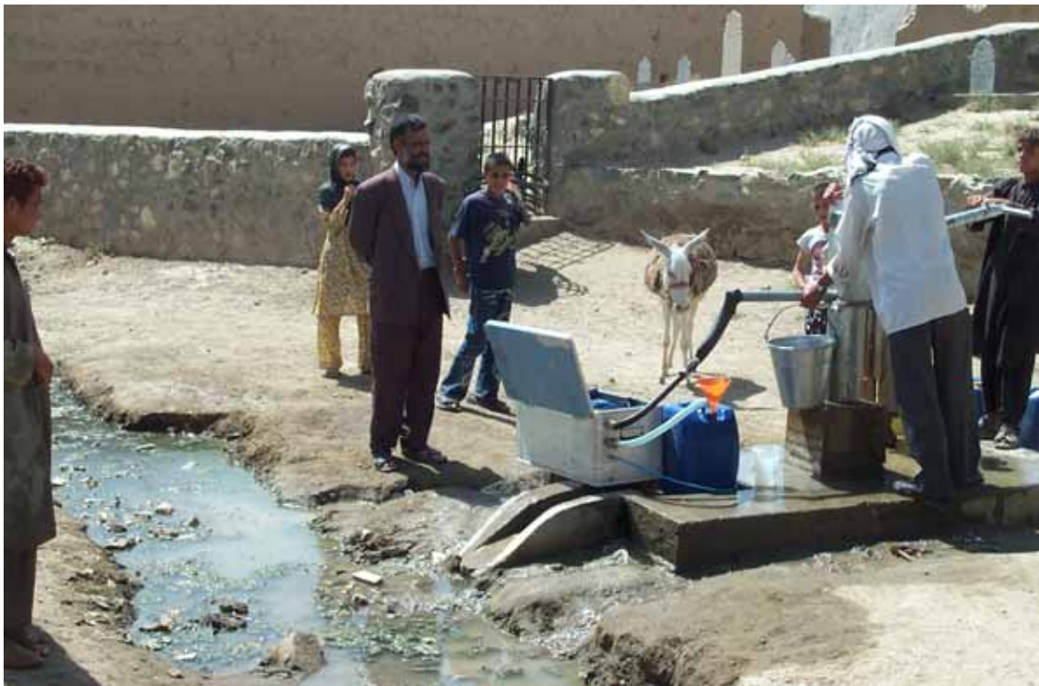
Fig. 3.63: A hand-pumped well extracting shallow groundwater in an urban district of Kabul immediately adjacent to an open sewage channel (photo: TÜNNERMEIER).
