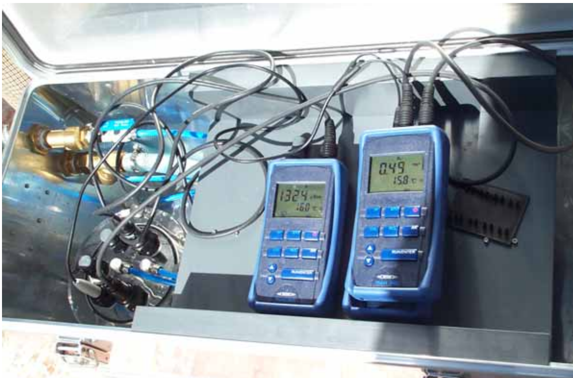
Fig. 2.3: Measurement of onsite parameters in pumped water using electrodes in a flowthrough cell (photo: TÜNNERMEIER).
