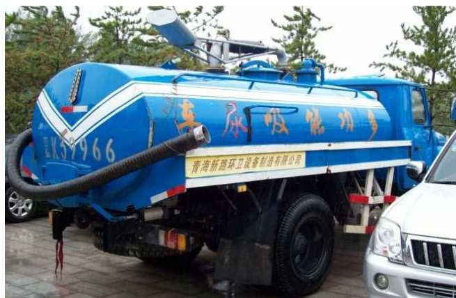
Fig. 5: Tanker truck to empty the urine tanks (source: Olt, 2008).
