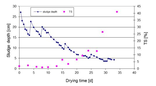
Decrease in sludge depth and increase in total solid content as measured in sludge drying beds
