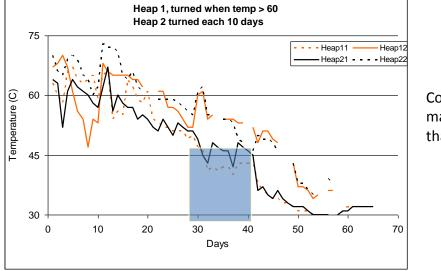
Co-composting process allowed to maintain temperature at > 45°C for more than 30 days
