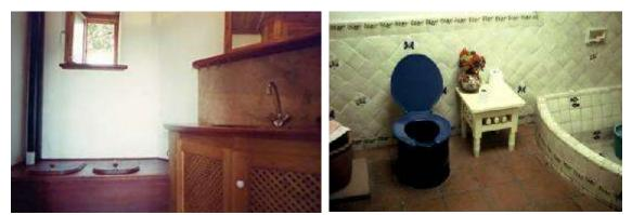
Figure 10: Dry toilet integrated into a bathroom. Source: www.rinconesdelatlantico.com
