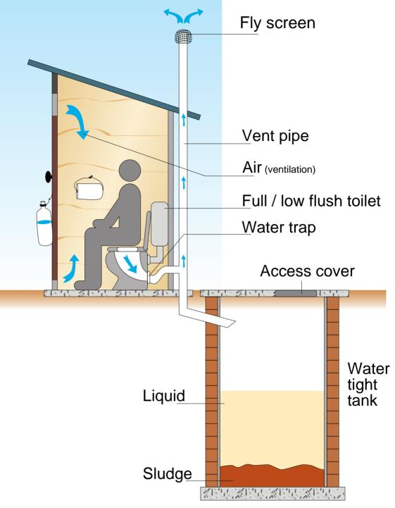
A storage system, i.e. a sealed tank, where low-flow or full-flush toilet systems are used.
