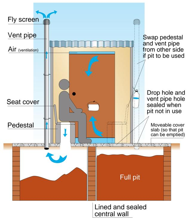
A single top-structure over 2 shallow pits, side by side. Only one pit - vented by a pipe protected with a fly screen - is in use at any time. Generally lined and the central wall fully sealed to ensure isolation of one pit from the other.
