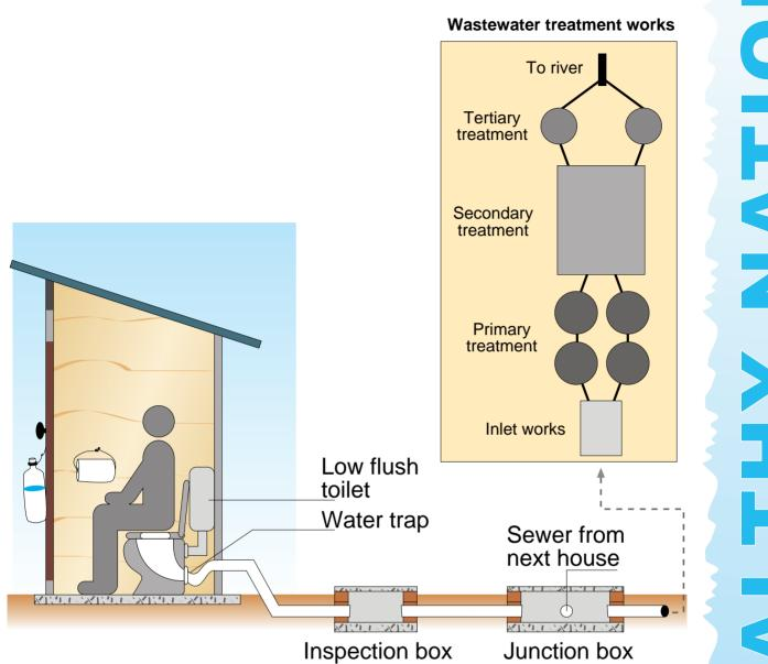
A toilet, usually in-house, flushed using lower volumes of water than either conventional sewerage or septic tanks, to smaller diameter sewers laid at flatter gradients and shallower depths between dwellings on a block. On-site shallow inspection chambers are provided.
