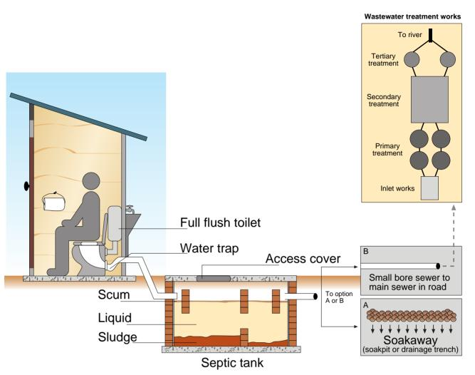
Septic tank and soakaway: An in-house full flush-toilet connected via pipe and plumbing fixtures to an underground watertight settling chamber (the 'digester') with a liquids outlet to a subsoil drainage/soakaway system.
