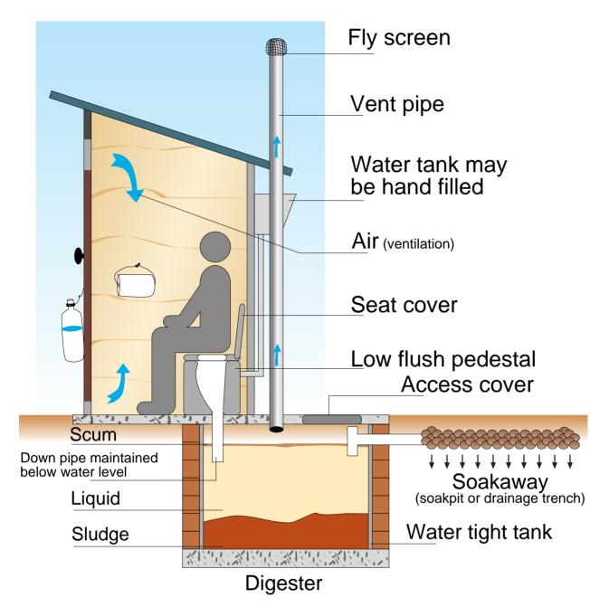
A toilet with a water-seal arrangement: a straight or curved chute running from the seat to below the water level with some form of waste collection and disposal system.
